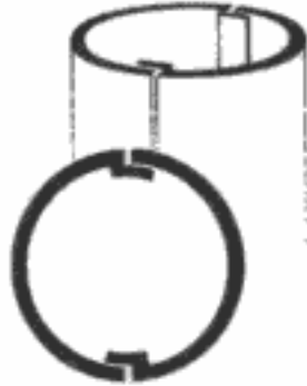
Lap Joint FILLED & FINISHED JOINT FOR SEAMLESS COLUMN FIELD PAINT AS DESIRED
